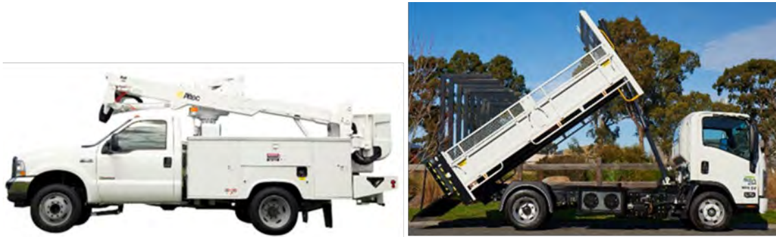
Figure 24: Images of Trucks Equipped with a Power Take-Off
